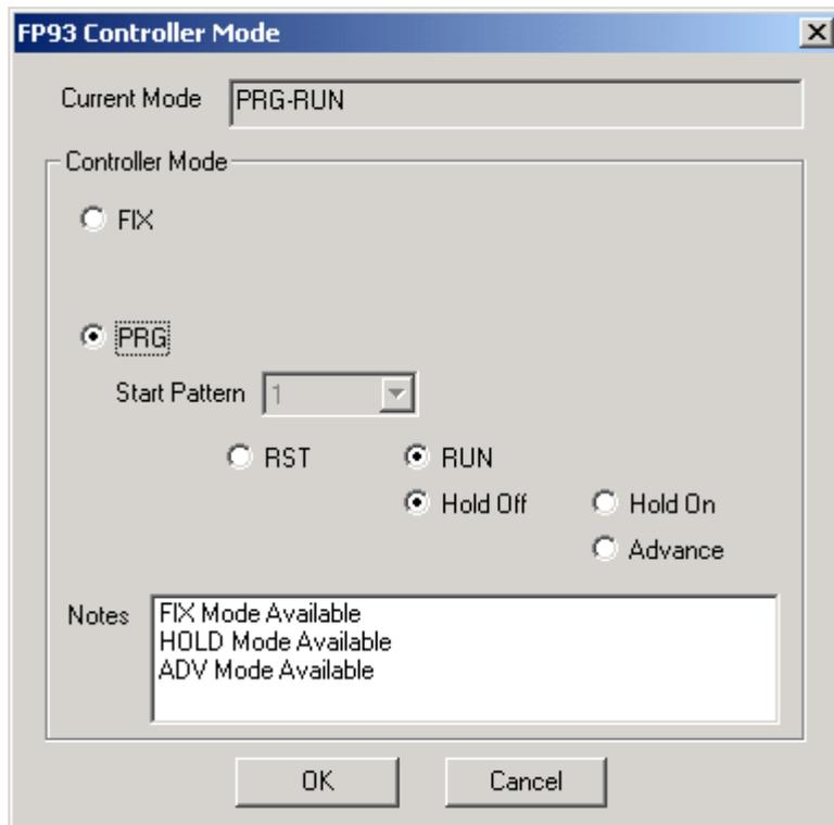
The controller is in pattern mode, click RST to stop the pattern, RUN to start it.
