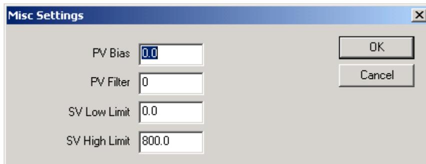
Enter the values for PV Bias and Filter and SV Limits, Click OK to write the data to the controller.
