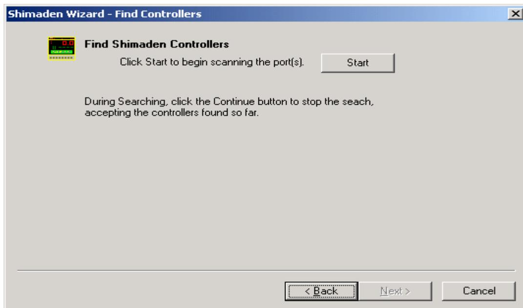
Click Start to begin scanning the controllers. As they are scanned, a Progress window is displayed.
