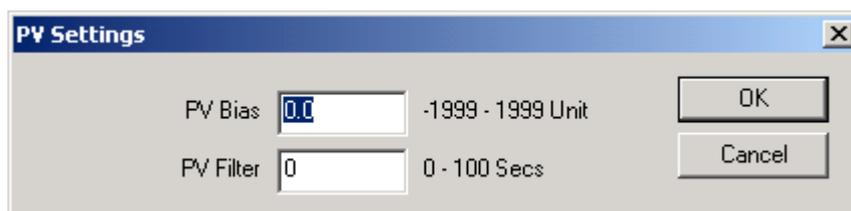
Enter the values for PV Bias and Filter, Click OK to write the data to the controller.
