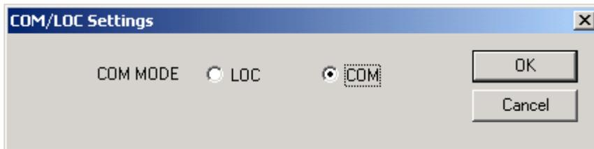
Click COM to put controller into COM mode, LOC to put controller into LOCAL mode. Click OK to write data to the controller.
