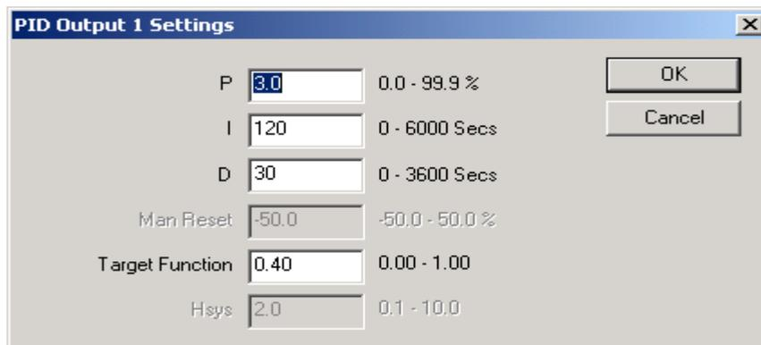
Enter the PID parameters as required, Click OK to write the data to the controller.
