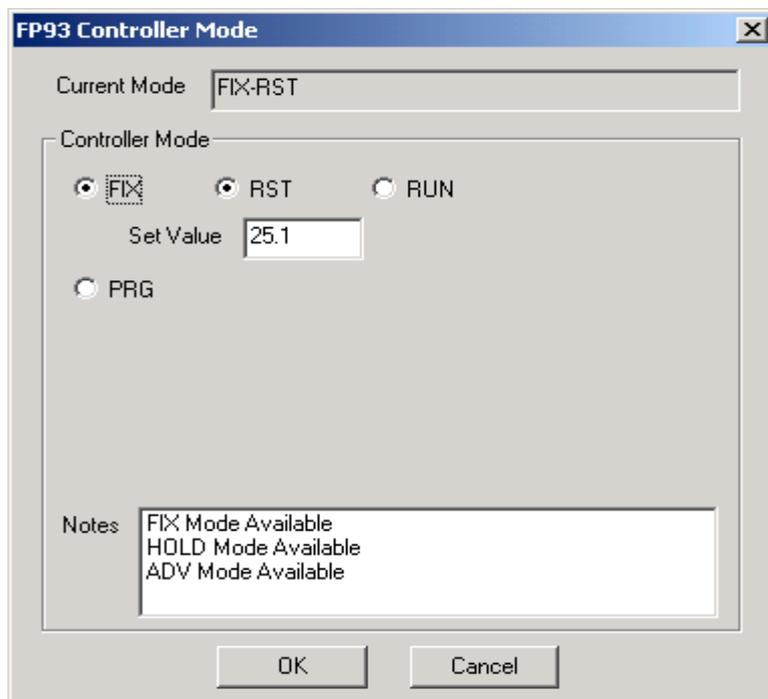
The controller is in FIX mode, click RST to stop the control action, RUN to start it.
