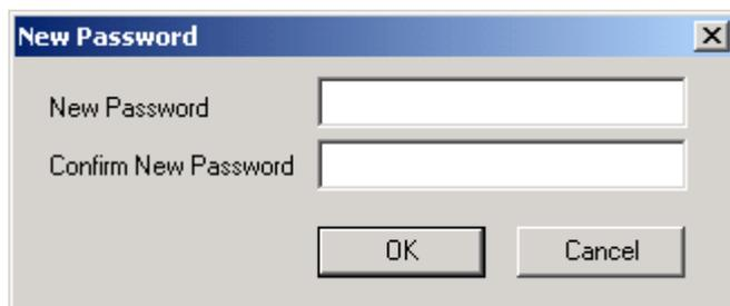
When “Use Password to close” is clicked, the program starts with the setups and buttons protected and a password must be entered to use them. When the setup password is entered, the button password is automatically set.
