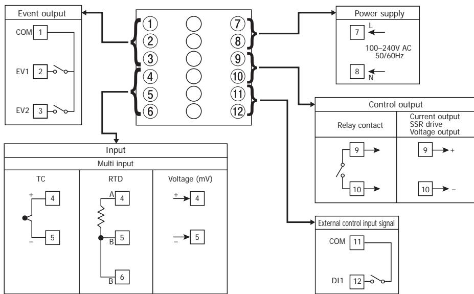
Crimp-type terminals fit M3 screws. Use crimp-type terminals that are no wider than 6.0 mm.
