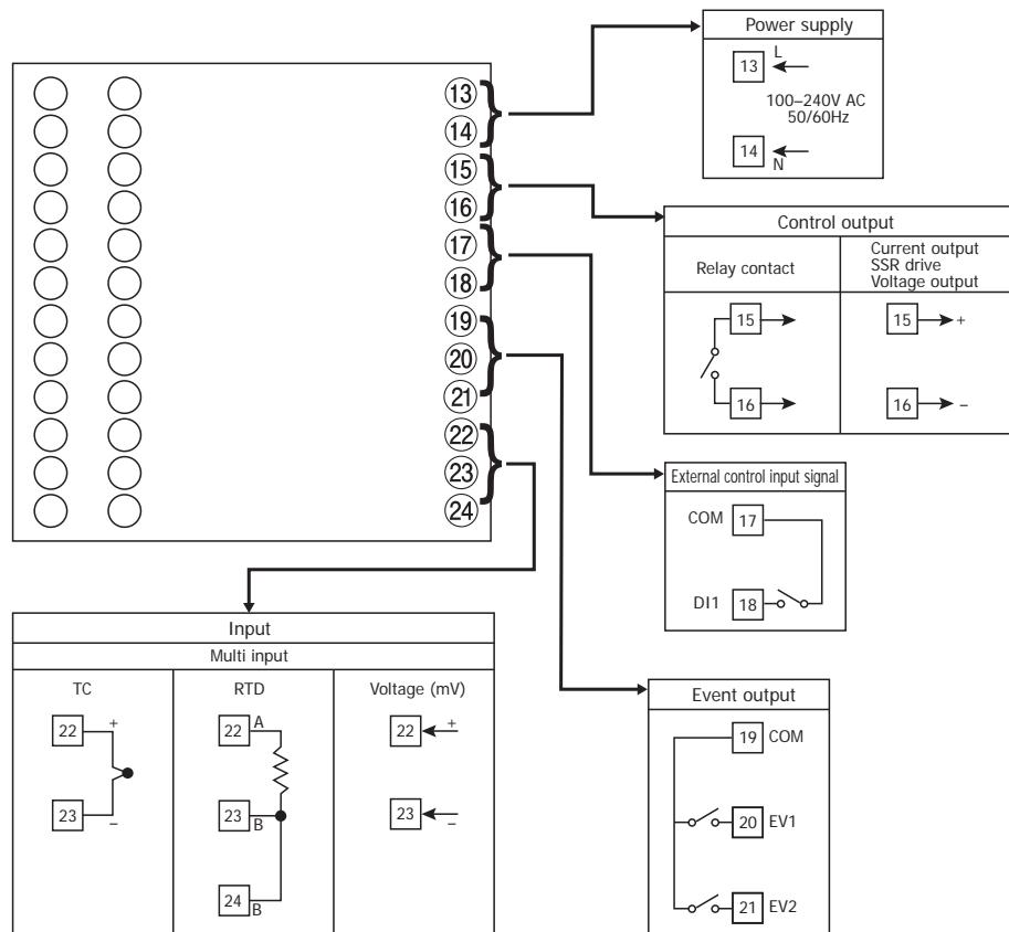
Crimp-type terminals fit M3 screws. Use crimp-type terminals that are no wider than 6.0 mm.
