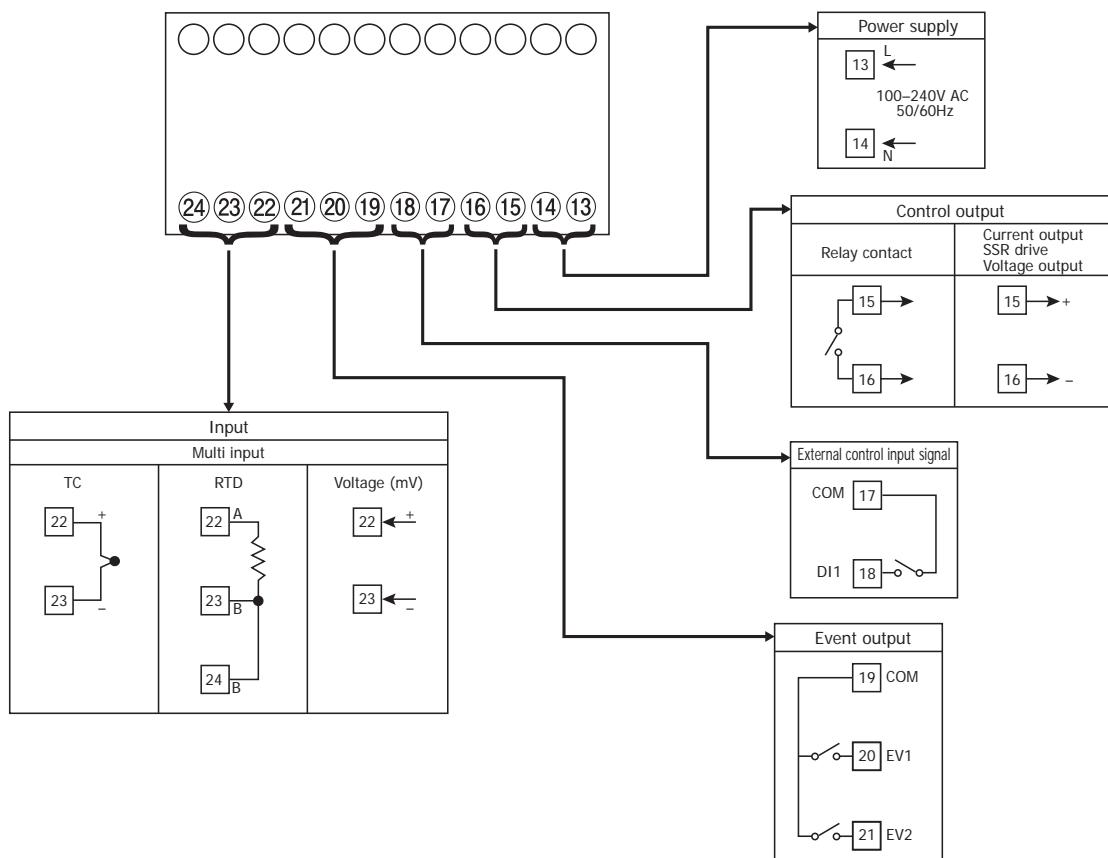
Crimp-type terminals fit M3 screws. Use crimp-type terminals that are no wider than 6.0 mm.
