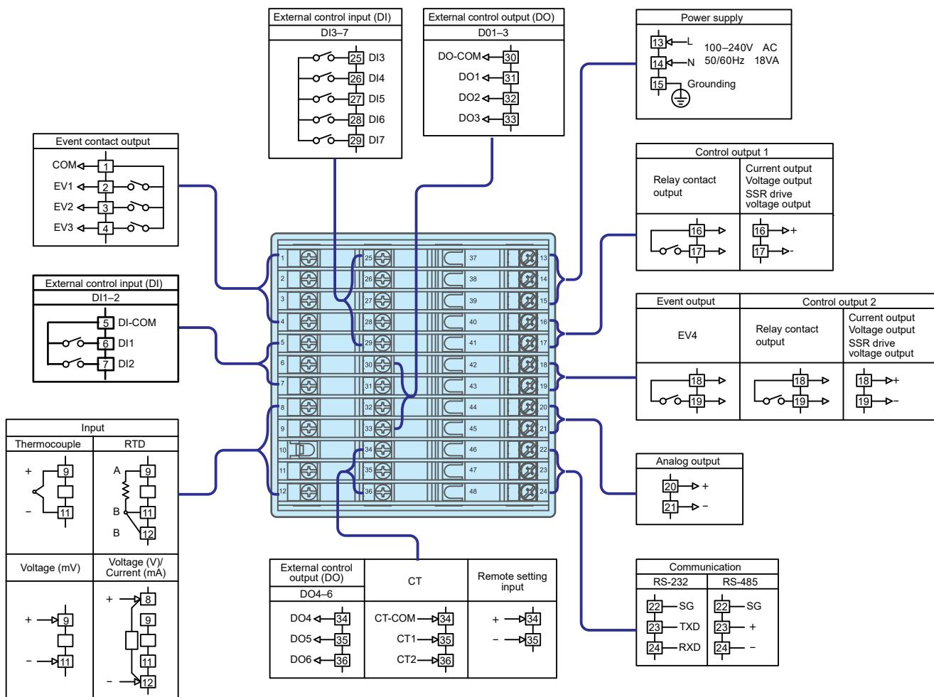
Terminal screw: M3 screw (No more than 6.2 mm width)
