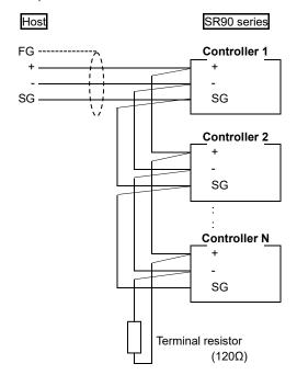
Note1: In the case of RS-485, provide it with the attached terminal resistor of 1/2W,  $120\Omega$  across terminals + and if necessary.
