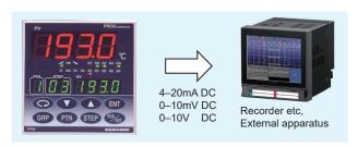
Communication function (option) Data communication to/from a personal computer, sequencer or the like can be performed by means of RS-232C or RS-485 signals.
