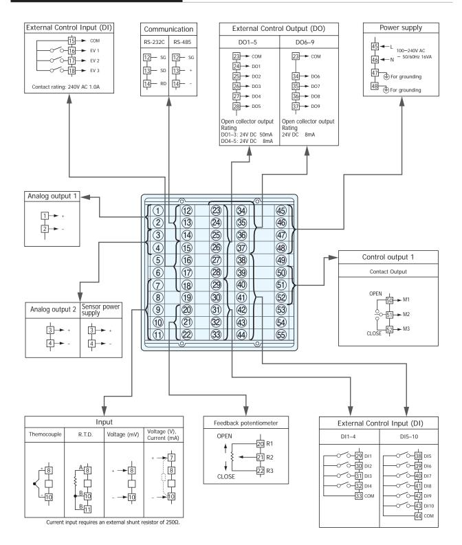
Crimp-type terminals fit M3 screws.
