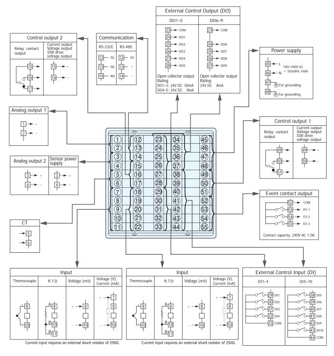
Crimp-type terminals fit M3 screws.
