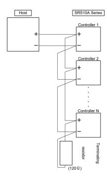
Note 1: With RS-485 specifications, you should mount the 1/2W 120 Ω terminating resistor that comes with the terminal element (between + and -) if necessary.
