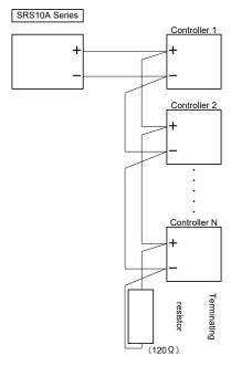
Note 1: With RS-485 specifications, you should mount the 1/2W 120  $\Omega\,t$  terminating resistor that comes with the terminal element (between + and -) if necessary. The terminating resistor should however be ultimately mounted on a single controller only. Operation cannot be guaranteed if a terminating resistor is mounted on more than one controlle
