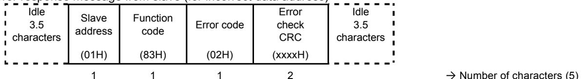
In a response message in case of an error, 1 is set as the most significant bit of the function code (83H).
