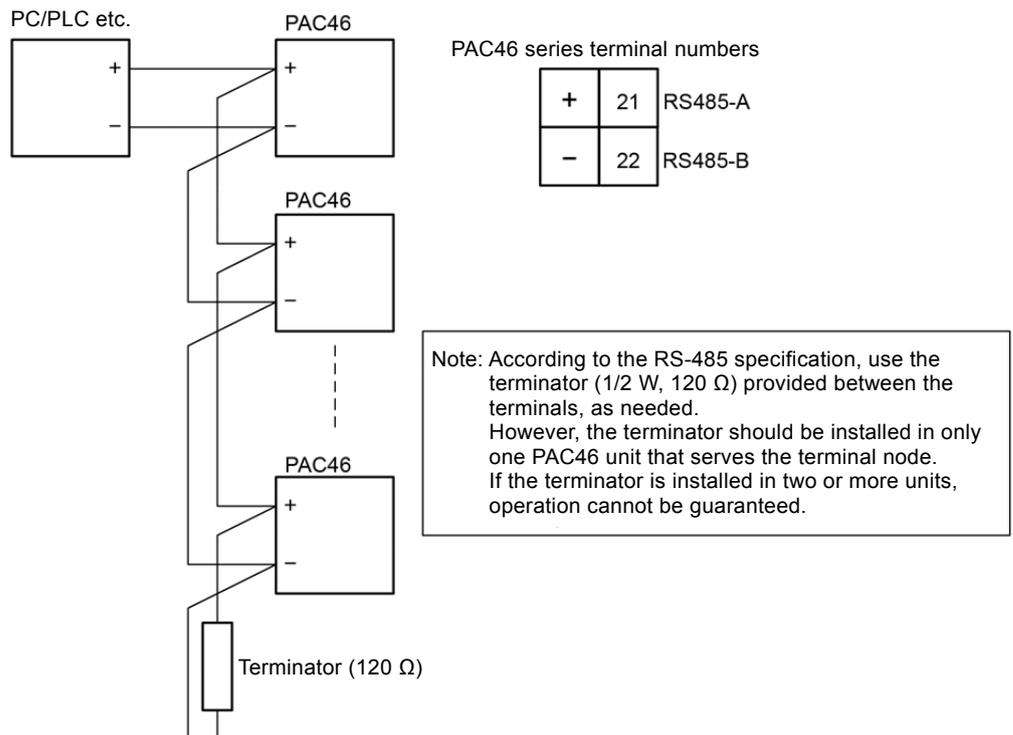
Note 4: If multiple units of the instrument are connected, you need to set a unique communication address for each unit.
