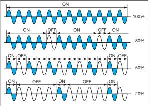
Cycle calculation zero voltage switching control system
