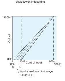
Example) Input/output characteristics diagram of
