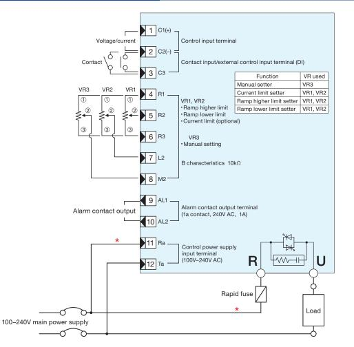
\*Note: Main circuit (power supply for loading) R terminal and the control circuit Ra terminal should be used in the same phase.
