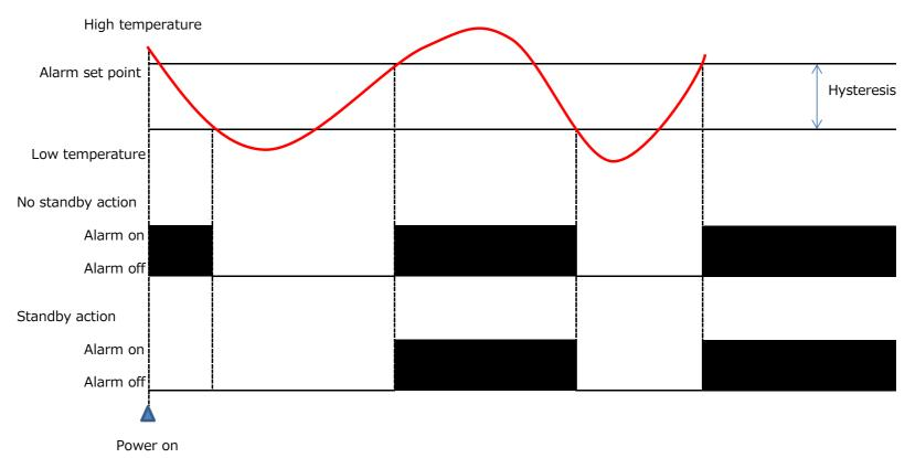
When power is applied, even if the measured value is in the alarm range, the device stands by without sounding the alarm. Once it exits the alarm range and enters the alarm range again the alarm sets off (there is only one time when the alarm does not sound, first time the measured value is in the alarm range).
